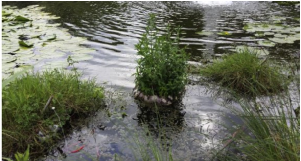
Floating Plant-MFCs by Schievano, A., Colombo, A., Grattieri, M., et al., (2017)
